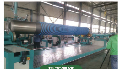
热态缠绕 Hot Winding
